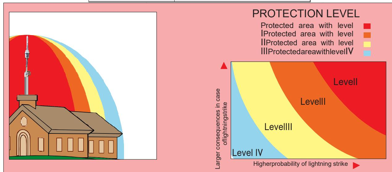
Accessing the risk of Lightning Protection System is based on lot of factors, however, it is recommended to opt Level I protection level.
