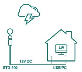
The BTD-200 lightning warning system is a modular system designed to operate out-of-the-box and is expandable as requirements grow or change. Its proven technology is currently used at airports worldwide and by national meteorological organizations.
